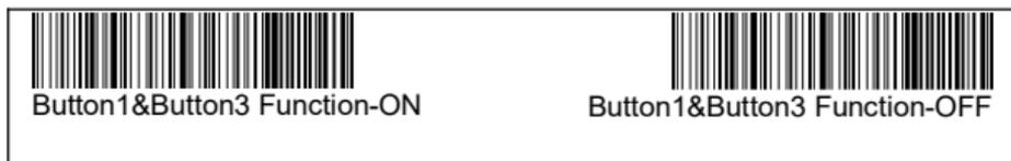
The functions of Button 1 & Button 3 are turned off by default, if you want to turn on, please scan "Button 1 & Button 3 Function-ON".
