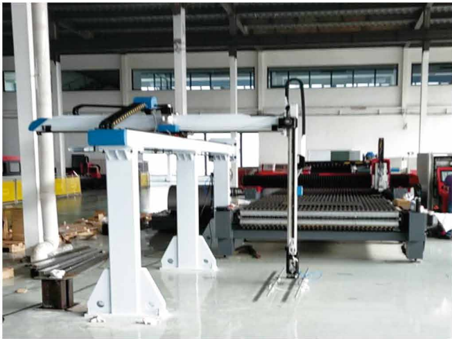
激光切割机后端下料、堆叠四轴牛头机械手 Four axis bull-head free style servo robot for laser cutting machine application
