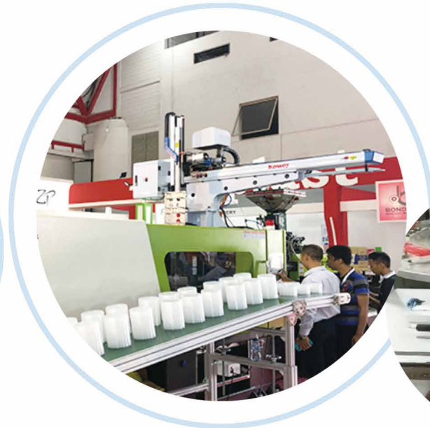
模外堆叠 Outside stacking
