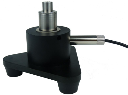
Figure 1 Photograph of the simulated ear
