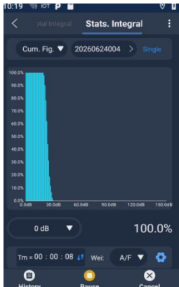
Figure 6-3-2-4 Cumulative Distribution Plot Interface
