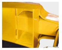
Extra reinforcement rod on top of the chassis. Leads to a longer chassis life time.
