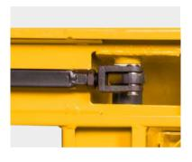
Adjustable push rod : Adjustable push rod design, after 1-2 years use, due to wrong load center, there might be situation with 2 forks not in the same even level, the customer can adjust the forks to even level with the adjustable push rod.
