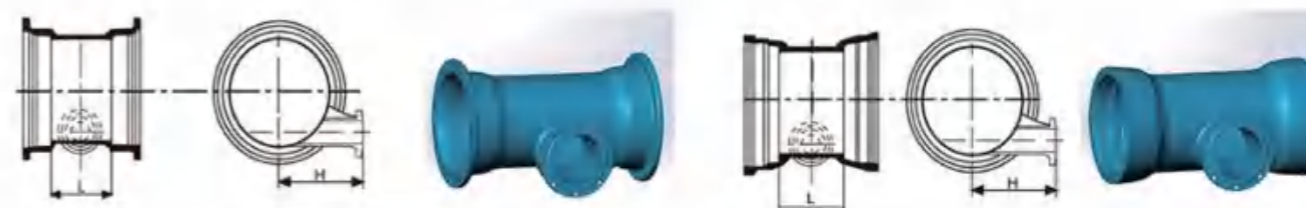
18 Double-socket level invert tees with flanged branch
