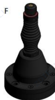
F NATO 4-hole Spring GPS Base L1 & L1/L2 GPS available 4 x M10 or 3/8" Bolts on 114mm (4.5in) PCD Base diameter 140mm (5.5in)
