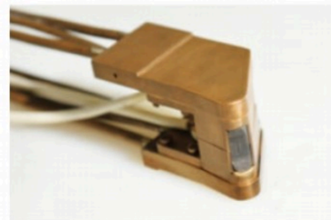
Ion source is pluggable and can be changed without opening the cyclotron body.
