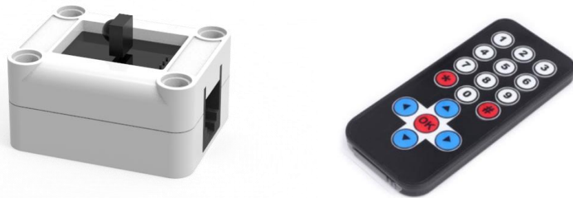
Infrared remote control receiving module (left), Infrared remote control board (right)
