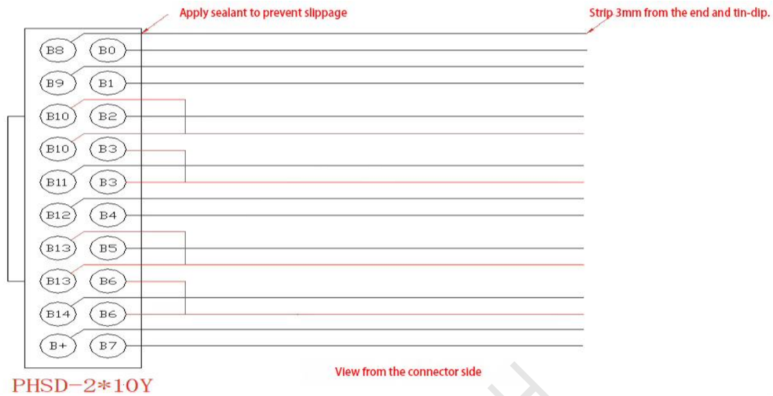
Figure 7-1: 14S Voltage Sampling Harness - Pin Assignment Detail
