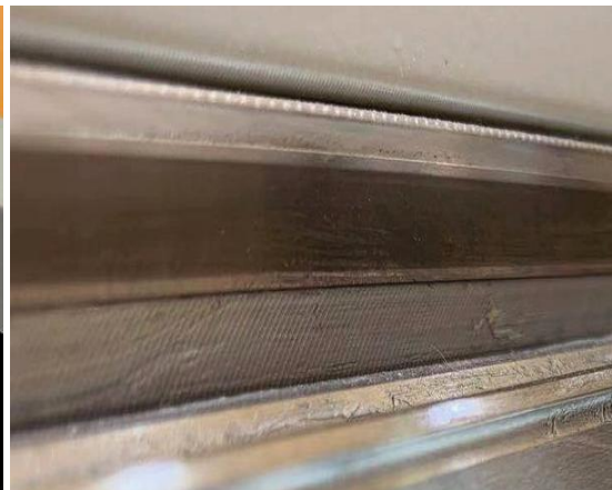
● Steel encoder for X-Axis high precision positioning.
