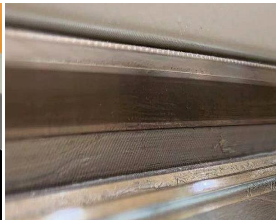
● Steel encoder for X-Axis high precision positioning.
