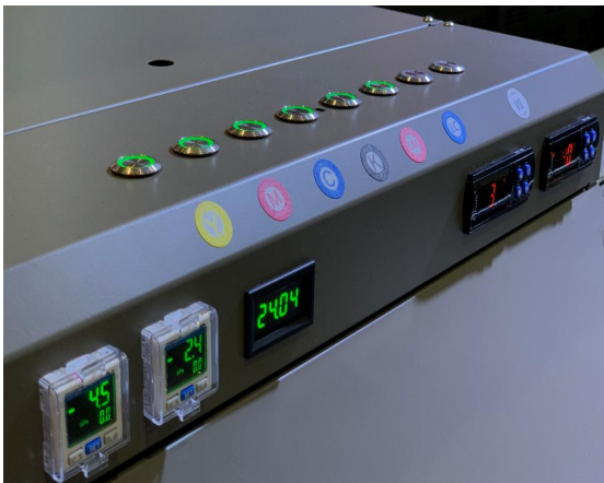
• Print head flushing control button+Temperature indicators+Negative pressure indicators.
