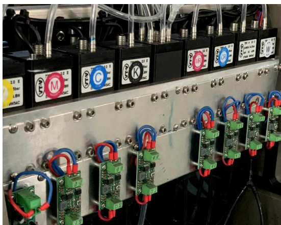
• Secondary Ink Tank Heating System
