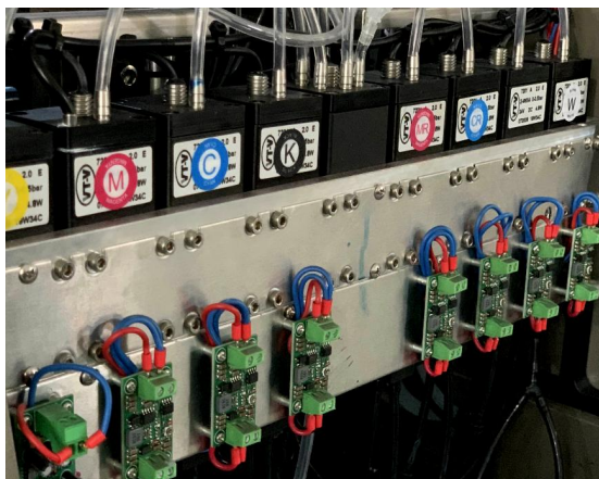
• Secondary Ink Tank Heating System
