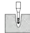
球头铣刀深沟加工 Ball nose end mills for deep slot machining
