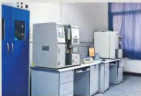
碳素测定仪及氧氮氢联测定仪 Carbon meter and oxygen nitrogen hydrogen meter
