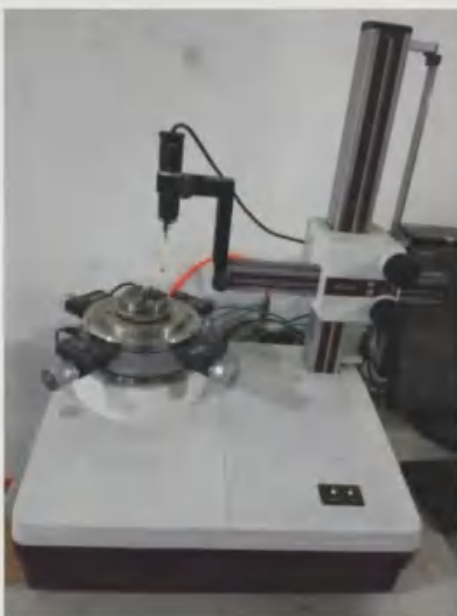
圆度仪 Roundness instrument
