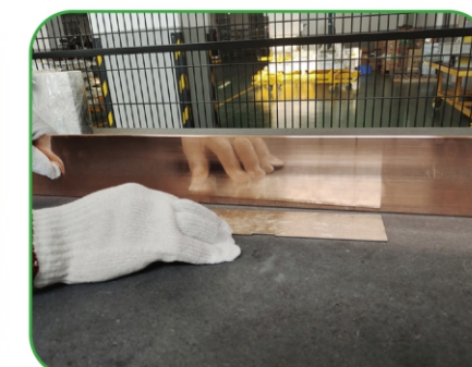
Flatness and Appearance Inspection of Copper Busbars
