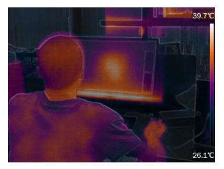
• Overlay fusion. The thermal camera overlay part of visible camera color, to let the background more clear, to identify the environment easily.
