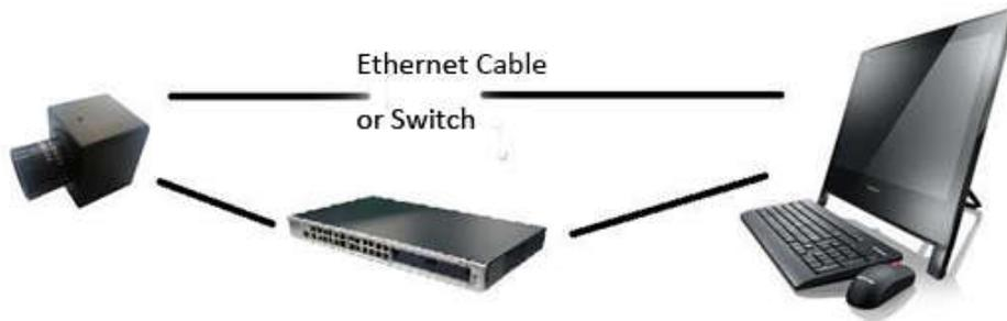
To connect infrared thermal camera with PC through Ethernet cable or switch, the IP address is "192.168.1.x", x is not the same as the camera, and the subnet is "255.255.255.0" Open the analysis software, to scan the camera in the left side, then connect the camera,
