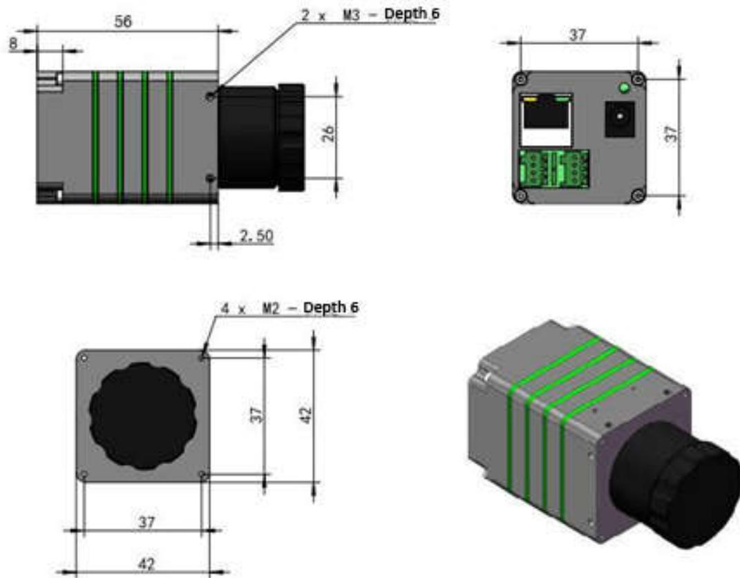
Figure: SR series dimension (mm)
