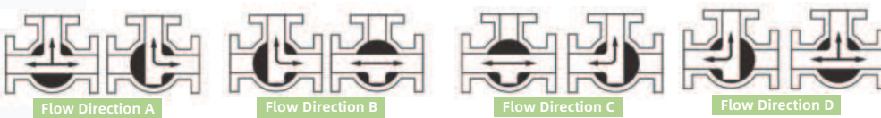
T-Pattern Flow Direction Diagram
