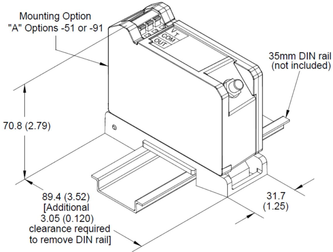
**Figure 16: DIN Mount 3300 XL 11 mm Proximity Sensor**
