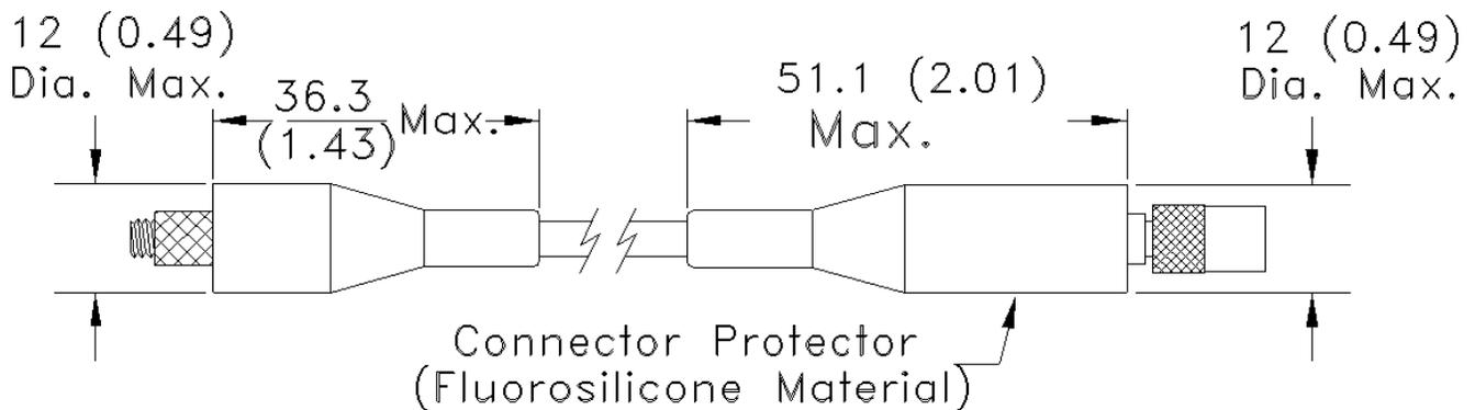
Note: Connector Protector only installed on female end when optioned. Both ends available as accessories.
