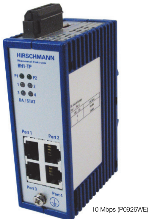
Figure 2. 4-Port, 10 Mbps (P0972WE) Ethernet Hub
