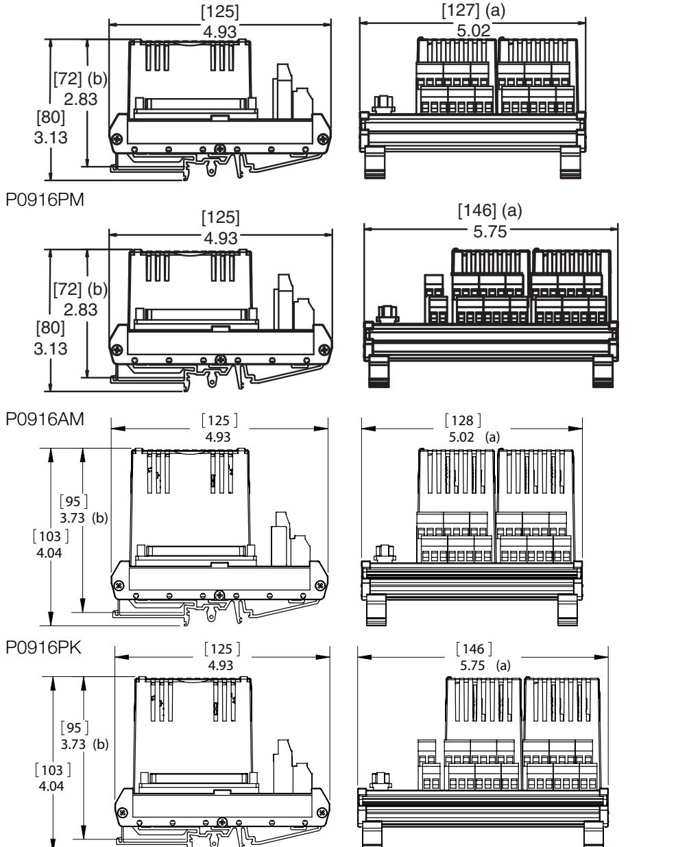
(a) Overall width – for determining DIN rail loading.
