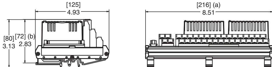
(a) Overall width – for determining DIN rail loading.
