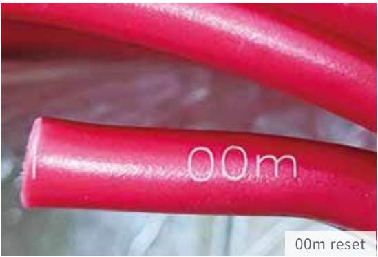
Connect to coiling machine meter mark speed 900 m/min
