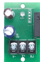
Battery under-voltage module (optional)
