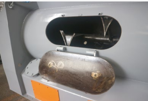
安全便捷的清理口 Cleaningout port with safe and easy access 打开清理口时设备不能运转 Stop machine once the port is open
