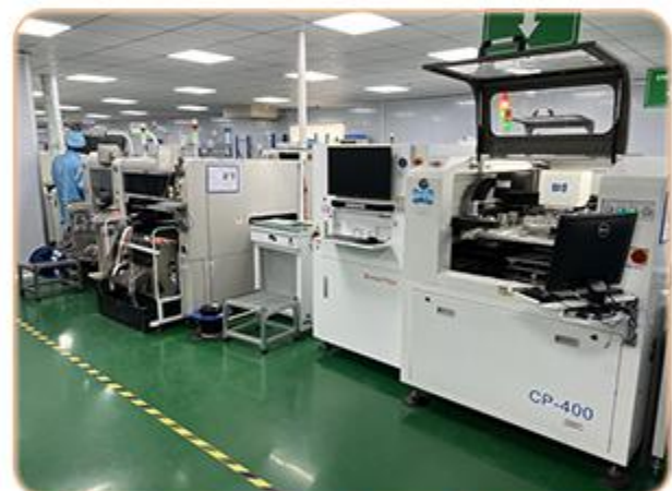
Automatic Solder Paste Printer with 3D Solder Paste Inspection System
