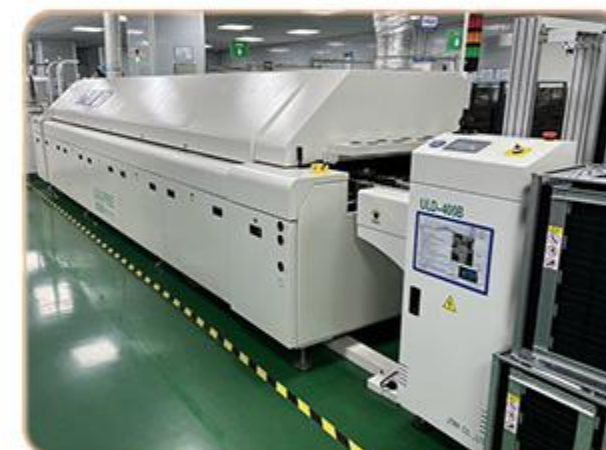
Reflow Oven with Fully Auto PCBA Unloader
