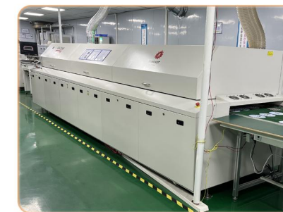
Lead-free Reflow Oven
