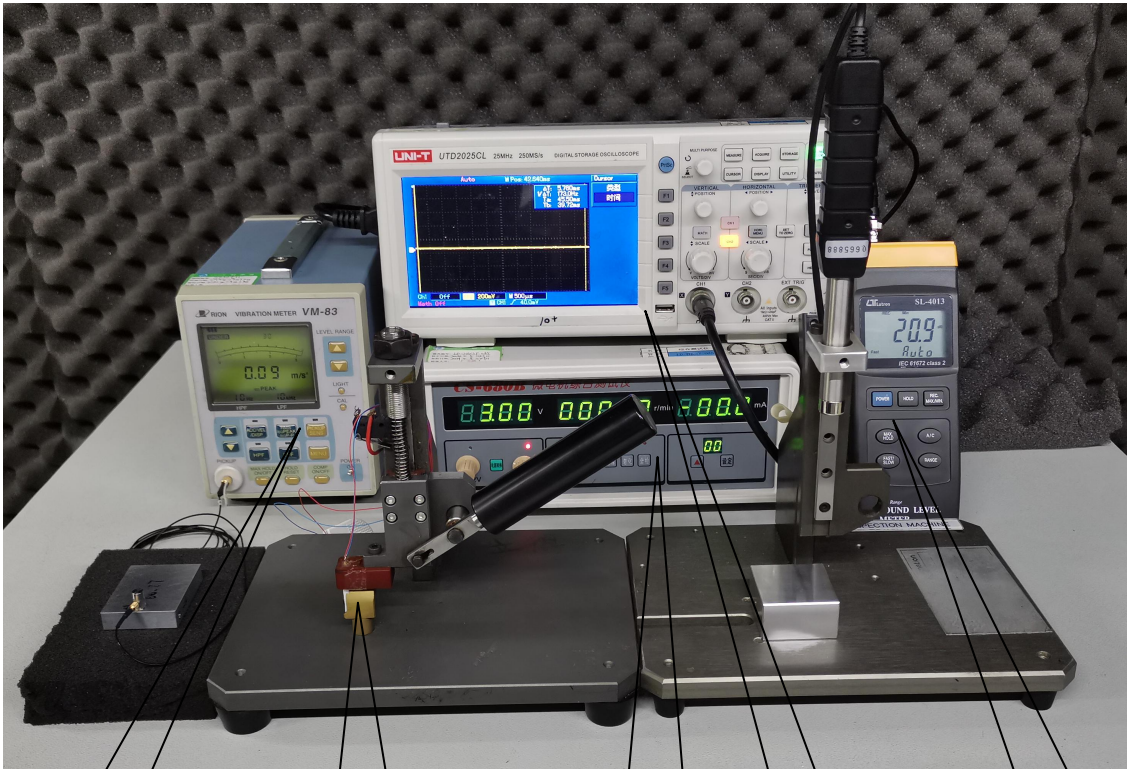
马达安装装置 Test Jig (for Clamping he Motor in Place)
