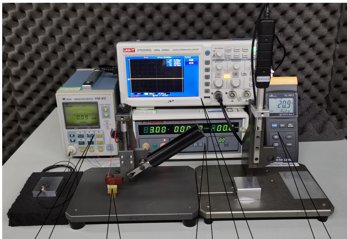
马达安放装置 Test Jig (for Clamping the Motor in Place)
