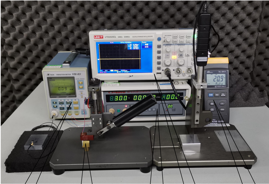
马达安放装置 Test Jig (for Clamping he Motor in Place)
