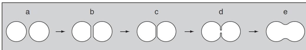
Deaeration improves drainage because the path length of the liquid from the mat to the filtrate tank. In a slurry saturated with bubbles, the liquid which drains from the fibers is required to travel in a crooked line downward, around all the bubbles in its way. By combining the bubbles into flocs or unstable large bubbles, the cumulative pathway from the mat to the filtrate tank is shortened and drainage rate increases.
