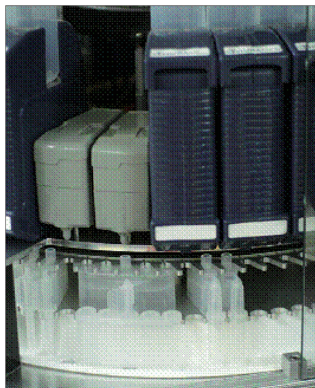
Schematic diagram of the main components of the instrument: injection station, emptying station, built-in reagent bottles, and large and small reactors.
