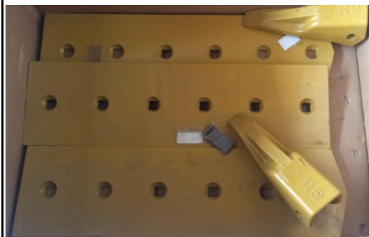
SEM822 Auxiliary blade plate ( 5202005 I+5202006 II )
