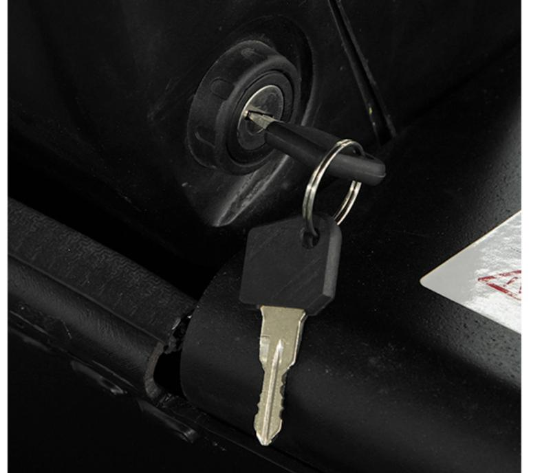
Fitted as standard, the key switch is water and vibration proof which makes it suitable to operate in cold storage applications.
