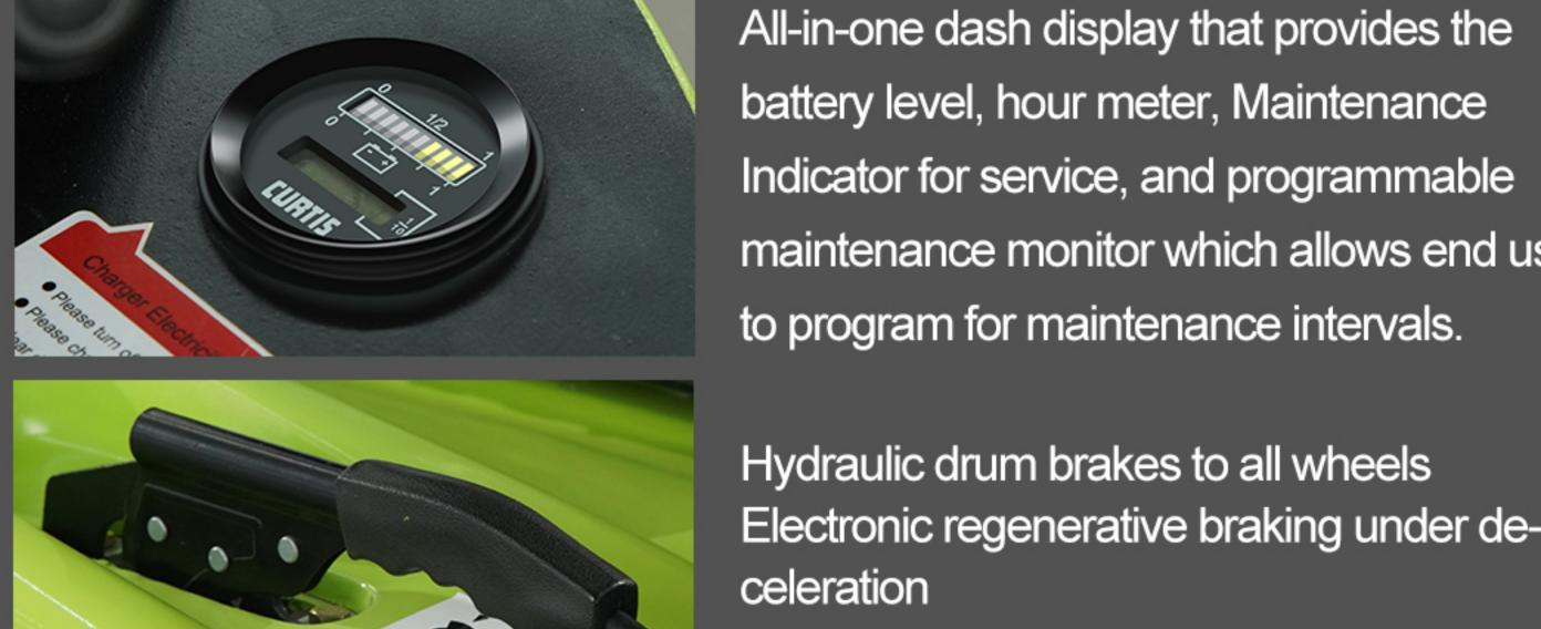
battery level, hour meter, Maintenance Indicator for service, and programmable maintenance monitor which allows end user to program for maintenance intervals.
