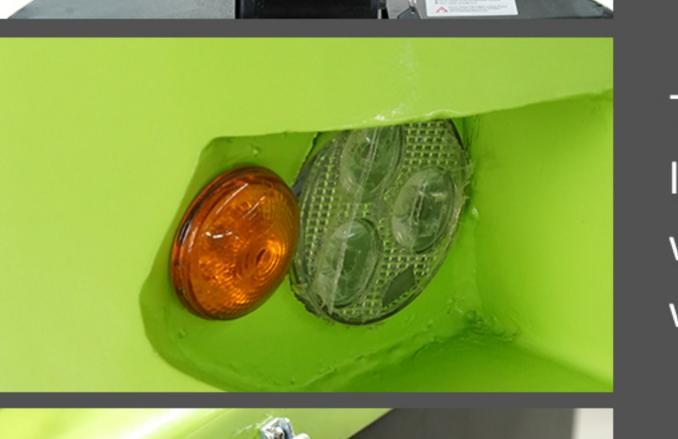
The QSD30/60 300 has headlight and stop/tail light as standard equipment. The headlight is wired to the key so headlight is on at all times with key on.
