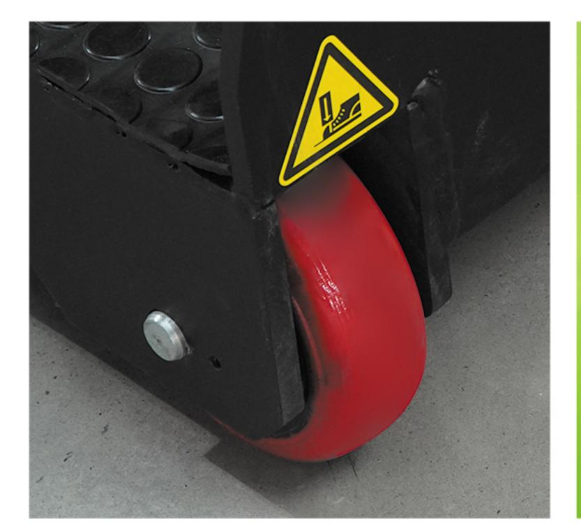
Both drive wheel & load wheels are made of polyurethane material with sturdy construction and high wear resistance that ensure better grip with the surface.
