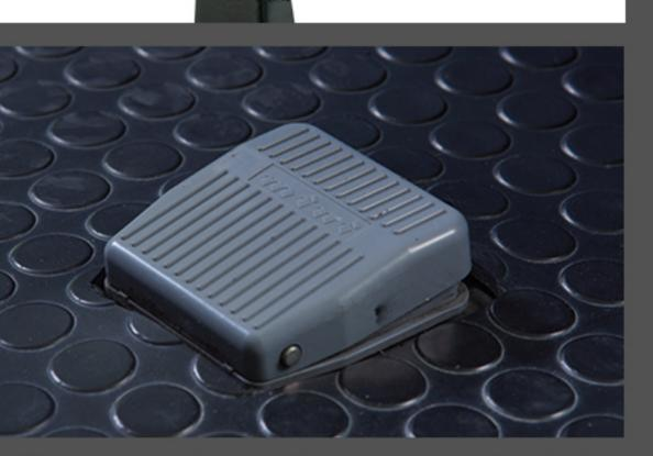
Safe pedal: when the pedal is released, traveling is stopped, and only hydraulic operation is enabled
