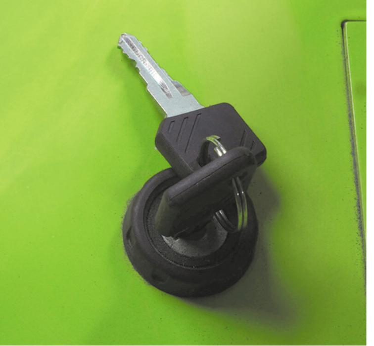
Fitted as standard, the key switch is water and vibration proof which makes it suitable to operate in cold storage applications.
