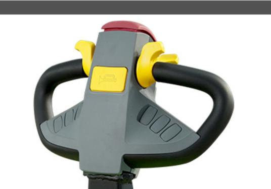
Multifunction control handle with ergonomically positioned handgrips for simplified operation of all controls with either hand.
