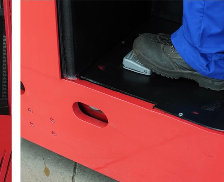
asy access to operator compartment with lower step design and the soft floor cushion reduces vibration and shock against operator.
