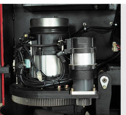
Control drive and hydraulic functions utilises integrated motor and drive motor are brushless making them virtually maintenance free.
