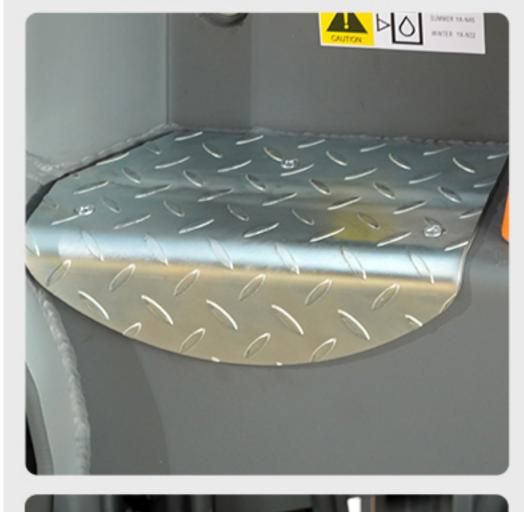
The two step pedal, the pedal is lower, the wider, the front column has the pull hand, facilitates the driver to enter the cabin, and leaves the spacious foot space.
