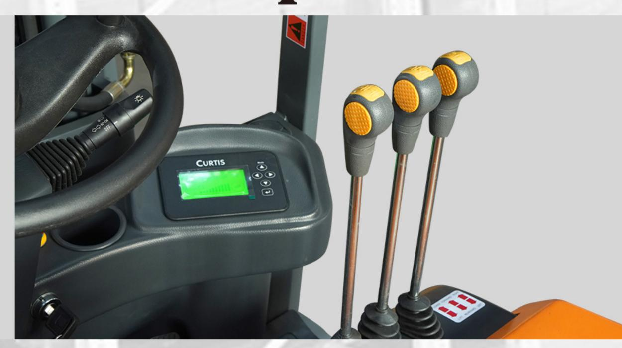
Three running modes to choose according to different needs: low speed, moderate speed and high speed.
