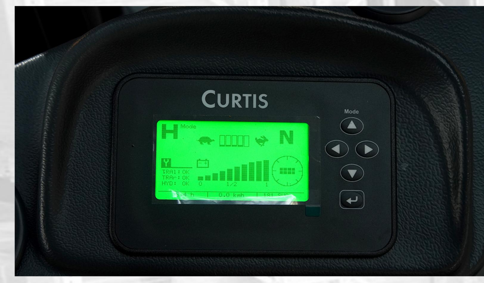
Mini electric forklift truck with import multi-function liquid crystal instrument, intelligent programmable LCD display, with fault code, electricity display, and various driving information.
