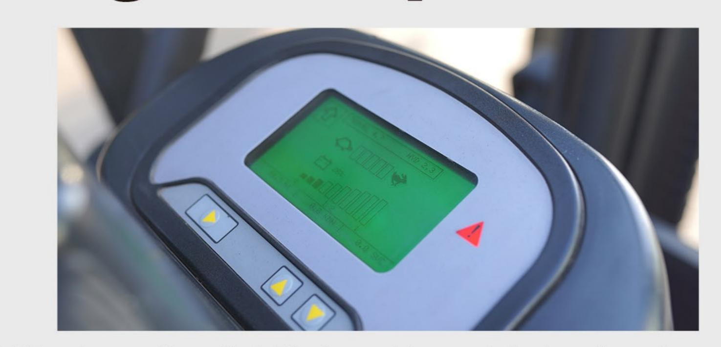
The LCD color monitor with 3.5 inch graphic smart display allows the operator to easily and efficiently control the machine. The monitor provides information about speed & accelerator level, steer angle & travel direction, battery discharge indicator, hour meter & working mode. The operator can select various performance modes to meet all working conditions.
