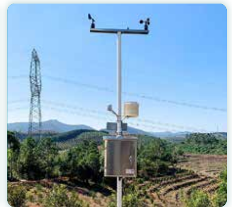
Field automatic weather station
