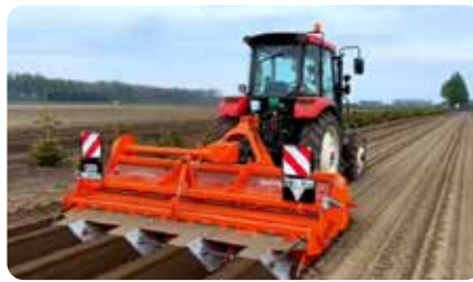
Ridge Making Operation
