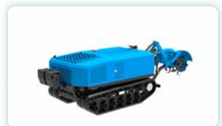
Unmanned trenching machine
