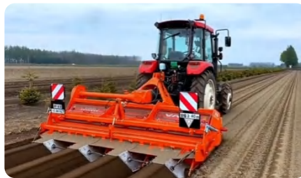
Ridge Making Operation
