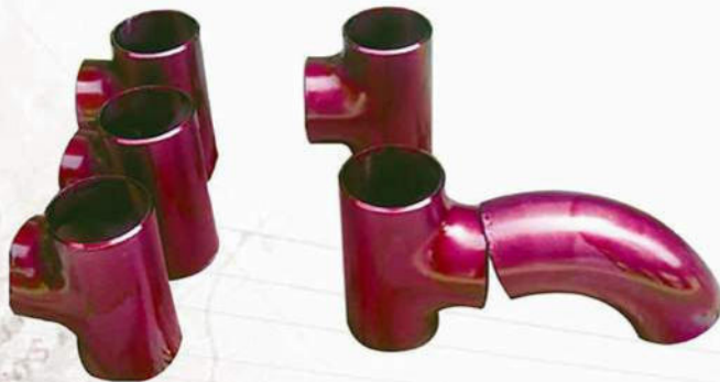
着色探伤 Crack Detection by Color
