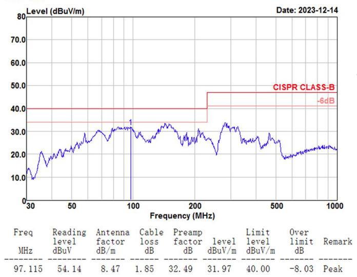
Radiation Interference Test (Horizontal)
