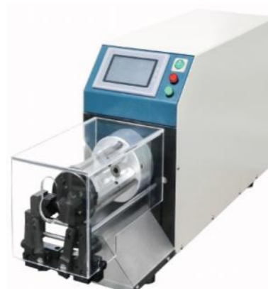
半自动剥皮机 Semi-automatic peeling machine
