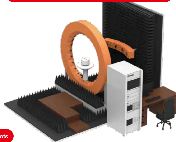
微波暗室：GTS 2200 microwave anechoic chamber x 2sets
