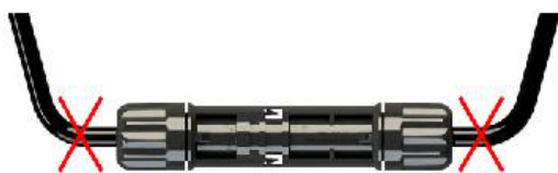
Wrong way for the cable
