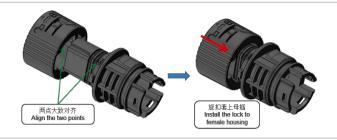
②沿箭头方向旋转卡扣"咔塔"一声后完成该装配; Rotate the lock in the direction of the arrow, finish the assembling after a "click" sound;
