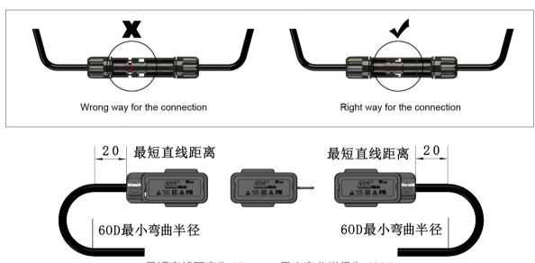
最短直线距离为 20mm, 最小弯曲半径为 6\*OD The minimum linear distance is 20mm and the minimum bending radius is 6\*OD
