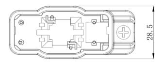
apply to 20SQ050; 30SQ050A; 40SQ045; Structure 4: y=4(28,5mm)
