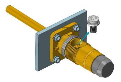
3.4 铆接端子的线缆插入插座壳体内 The cable of the riveted terminal is inserted into the socket shell
