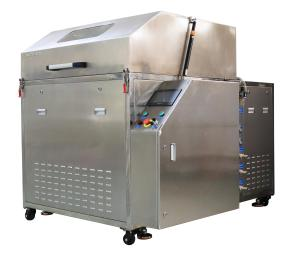
the surface of machine parts. The "spray cleaning machine" uses technologies such as high-pressure spray cleaning, high-pressure spray bleaching, high-pressure air cutting, and large flow fan hot air drying in the rotating basket to ensure the cleaning effect. The equipment is mainly composed of rack, spray cleaning
